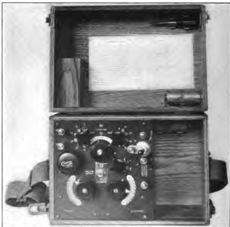
Plate 2. —Simple crystal detector receiving set having tuned primary and secondary circuits. Signal Corps set type SCR-54-A.
